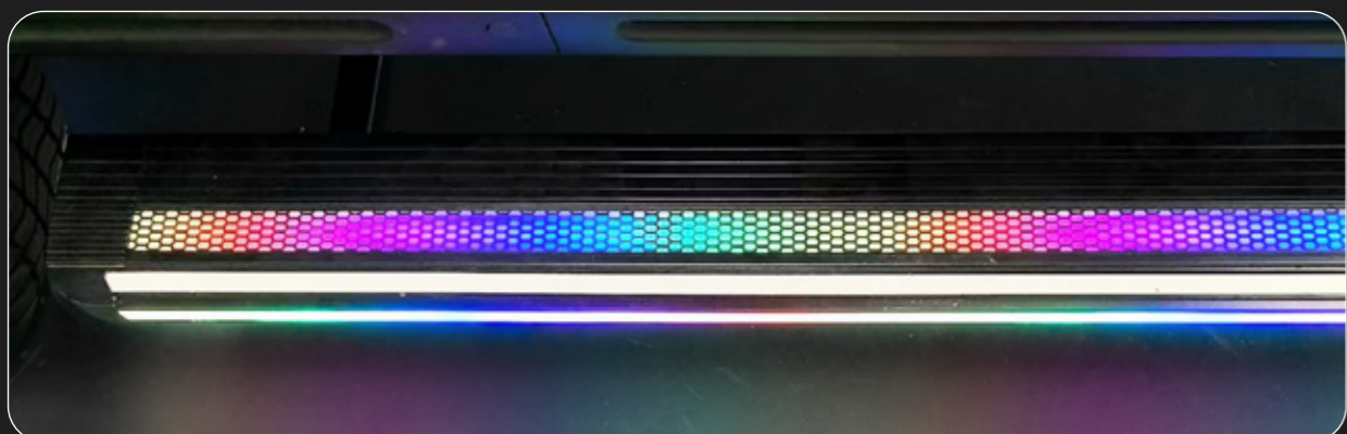
Running boards made of aluminium material and are equipped with ambient lighting.
